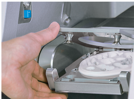
One-handed clamping made possible by DirectDiscTechnology
