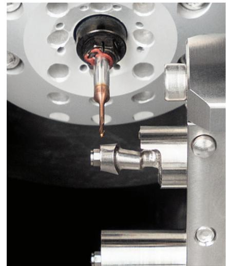
Most accurate milling of abutments
