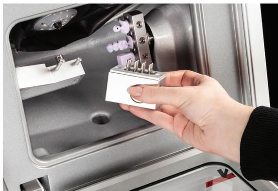
Inserting the tool magazine with one click
