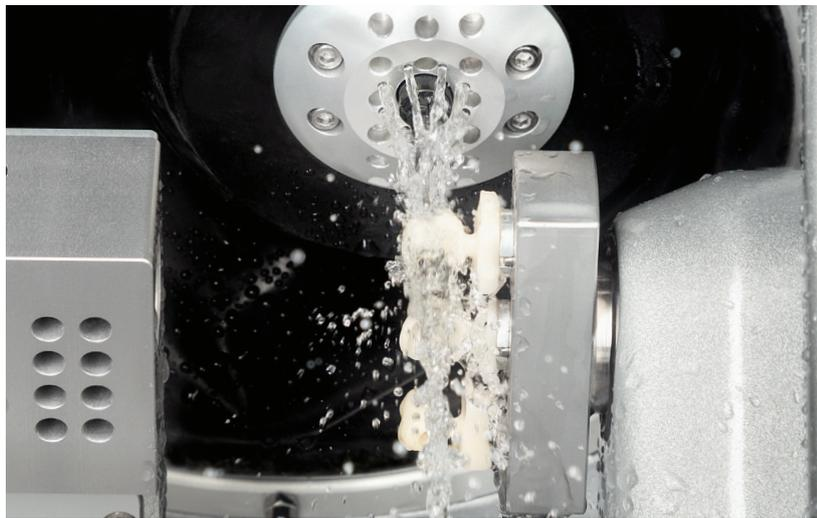
Highly precise grinding of glass ceramics or composites
