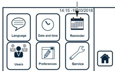
Select if and when the Test reminders (Vacuum - Helix/B&D - Vacuum + Helix/B&D) should be enabled, using the available options. Once the fields have been set, confirm with ENTER. Reminders activate at 8 a.m. of the selected day or upon switching-on (if it occurs after 8 a.m.).
