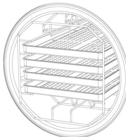
Or, if tray holder support is extracted and turned by 90°, it can be used to house special "boxes" (3/4 compartments based on sterilizer model).
