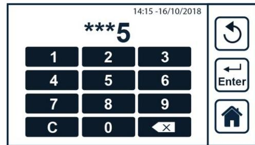
The ADMIN user can decide whether the sterilizer will ask for the generic user PIN at the cycle start (PIN Start) and/or at the end of the cycle (PIN End).
