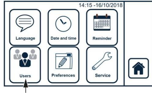
When using the device for the first time create the ADMIN user (identified by \*) following the indications in the figure on the side. Fill in the fields inserting ADMIN user name and PIN. Press ENTER to confirm.
