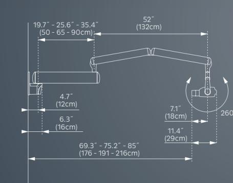
Note: Dimensions are based on single stud mount and short cone. Two-stud mount extends out an additional 1 3/4" (3.0cm)
