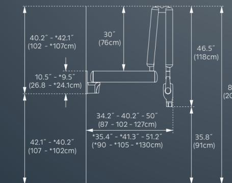
Note: Dimensions are based on single stud mount and short cone. \*Denotes dimensions based on two-stud mount.
