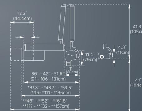
Note: Dimensions are based on single stud mount and short cone. \*Denotes dimensions based on two-stud mount oriented to the right. \*\*Denotes dimensions based on two-stud mount oriented to the left.
