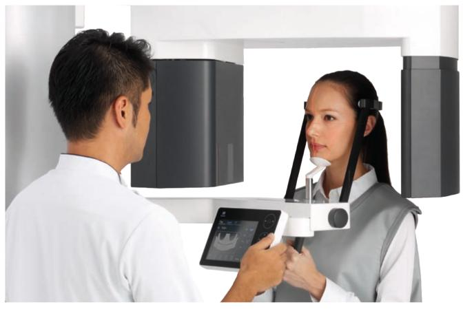
**Face-to-Face Positioning** Laser beam positioning is more accurate if you have good communication with the patient. Wheelchair Compatible The chin rest can be lowered to 865 mm (Short Column) to accommodate patients in wheelchairs.
