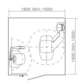
The unit must be fixed to the floor and wall when installed. If minimal layout dimensions are used, there may be very little space to move around inside the booth.
