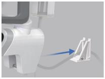
Pull out the holder backward and remove the main tube.
