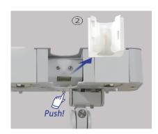
Remove it by pulling while pressing the lever.
