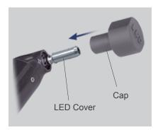
Put the cap on the LED cover before autoclaving.
