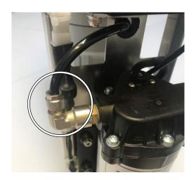
**13.** Cut the PUR hose approximately in the middle between the mixed-bed resin cartridges and the switchover valve.
