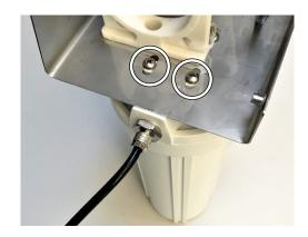
**10.** Lead the PUR hose of medium length through the recess to the pump.
