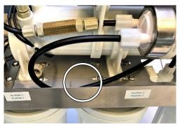
14. Insert the pressure switch at the point where it was cut.
